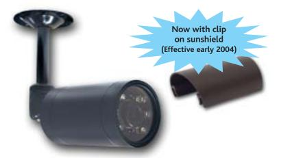
This completely waterproof B/W camera with built-in IR illumination is excellent for any indoor or outdoor application. The 1/3" CCD camera offers a 3.6mm lens, 420 lines of resolution and .02 lux sensitivity with 8 leds add CDS sensor for optimal viewing in extreme low light or complete darkness. This unit can operate under 90 feet of water and includes 60' of cable, mounting bracket and a 12V DC power supply. Also available in white housing with a 3' cable (CVC-320WP/W).
